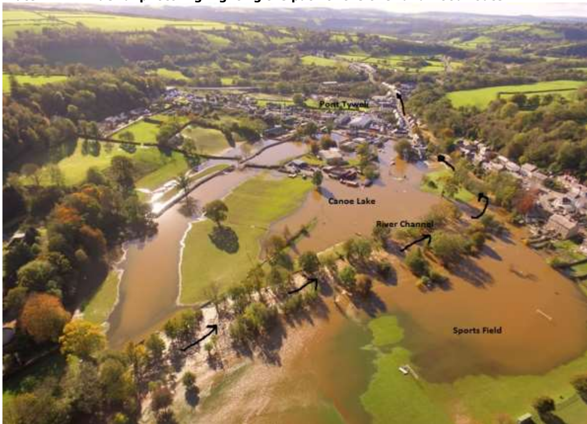
Plate 11 NRW aerial photo highlighting the path of the overland flood route.
